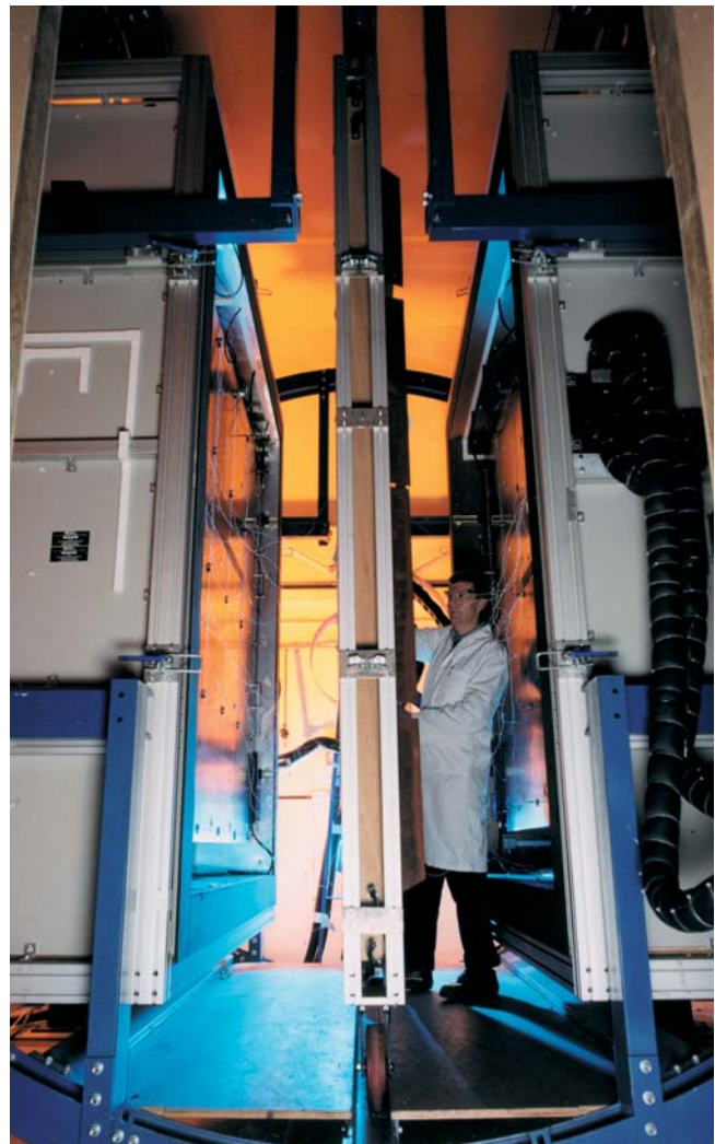
The National Physical Laboratory hot box apparatus provides an accurate method of measuring actual U-values for rooflights. It can be rotated into any orientation, enabling measurements to be carried out in the orientation that the product will be used.
