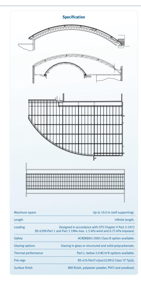
Illustrated here are details from an installation, designed and constructed with low-rise geometry.
