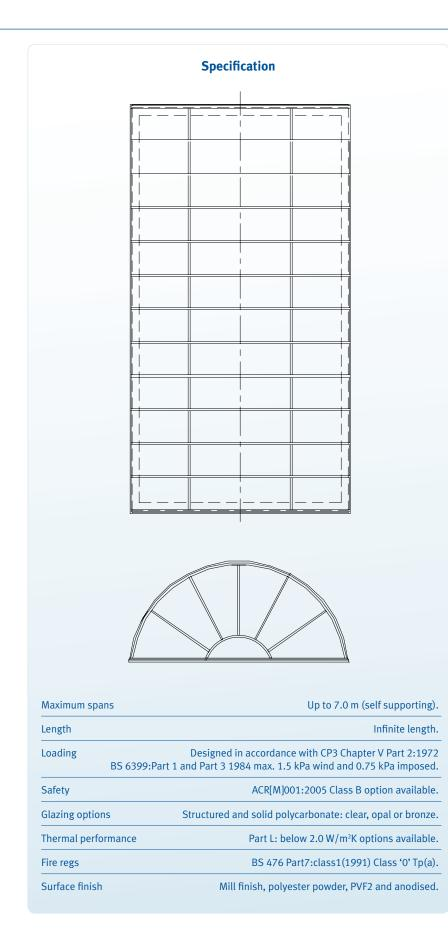
Illustrated here are details from an installation, designed and constructed with semi-circular geometry.
