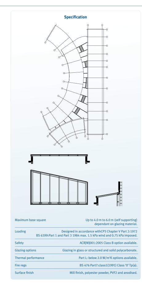
Illustrated here are details from a mono-pitched installation, designed and constructed with 15° geometry. Several such rooflights are arranged around a newly constructed building, introducing daylight to areas that would otherwise lack the benefit of natural light.
