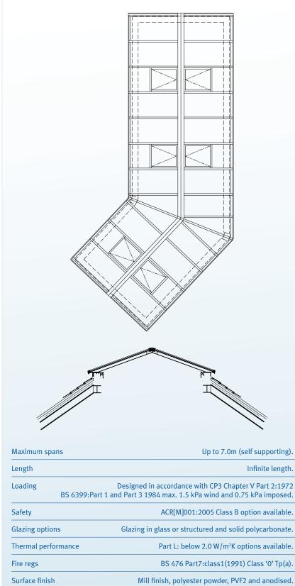
Illustrated here are details from a ridgelight installation, designed and constructed with 30° geometry and surmounting a pitched roof.
