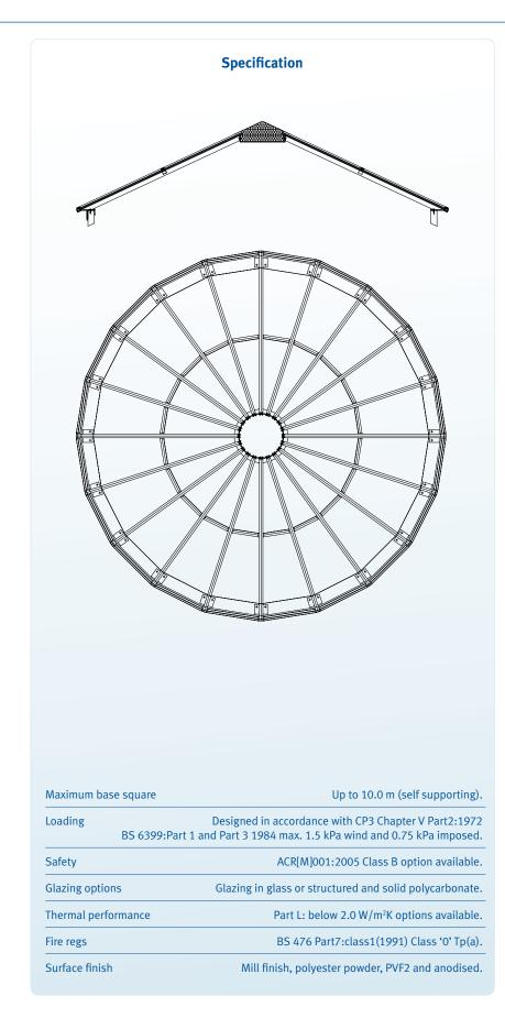
Illustrated here are details from a selfsupporting pitched polygon installation, designed and constructed with 30° geometry and set into a sloping metal profiled roof.
