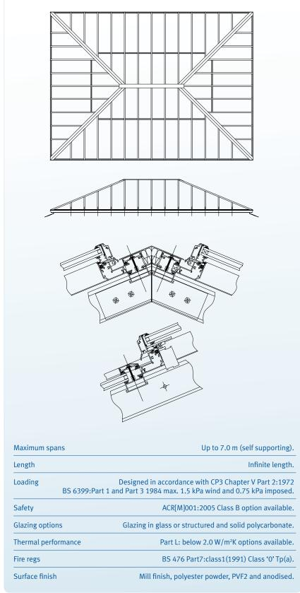
Illustrated here are details from a hippedend ridgelight installation, designed and constructed with 30° geometry.
