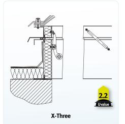
Thermally broken metal system with a U Value of 2.2, 'glazed' with either double glazed glass, triple skinned polycarbonate or solid finish. Metal frames and kerbs are white as standard, coloured on request.
