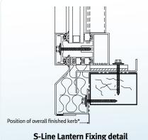
\* Please note the size refers to the overall finished kerb size including weatherproofing.
