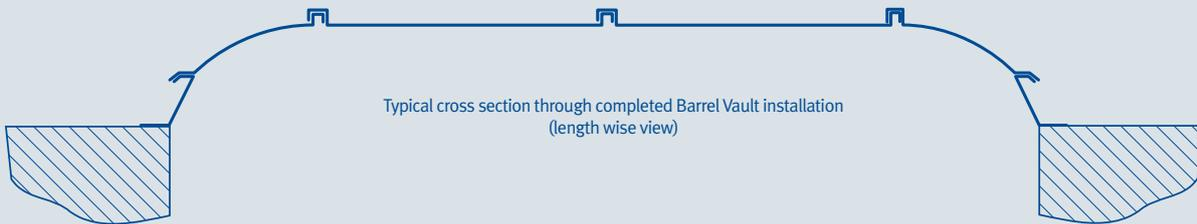
Typical cross section through completed Barrel Vault installation (length wise view)
