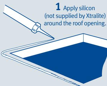
**1** Apply silicon (not supplied by Xtralite) around the roof opening.
