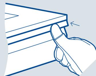
**8** Attach the ventilation zone. It will clip into the attachment zone with a 'click' when it is properly located, pressure can be applied to the top of the ventilation zone using your knee.
