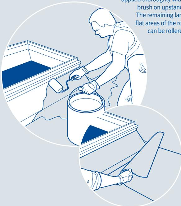
The adhesive needs to be applied thoroughly with a brush on upstands. The remaining large flat areas of the roof can be rolled.
