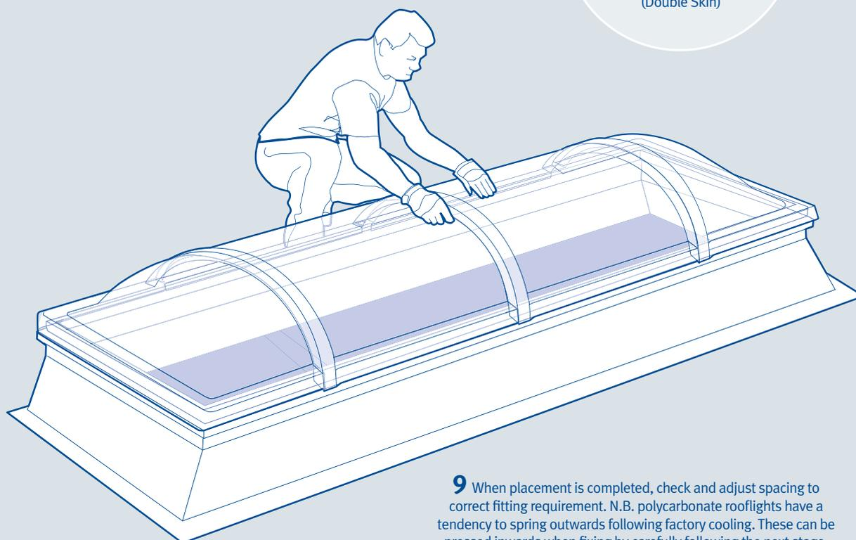
**9** When placement is completed, check and adjust spacing to correct fitting requirement. N.B. polycarbonate rooflights have a tendency to spring outwards following factory cooling. These can be pressed inwards when fixing by carefully following the next stage.
